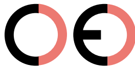
False CE Mark (too far)
